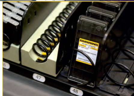
Spiral modul for single item dispensing, actually for single unpacked inserts.
