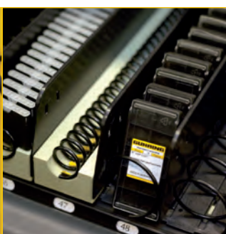
Expansion module spiral machine: Multi-supplier capability with drawers for restricted access when stocking. Single dispensing is possible with separate flap.
